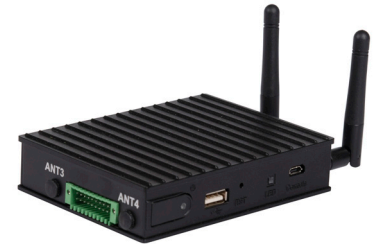
Easy-to-use push-fit connectors for sensor connection included.
